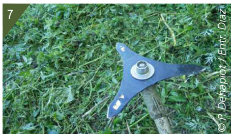
6. A shredder blade and the results in the field. 7. A cutter blade and the results in the field.
